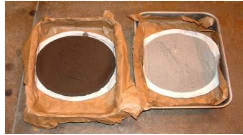
Figure 3-1. Quartz and Magnetite samples
